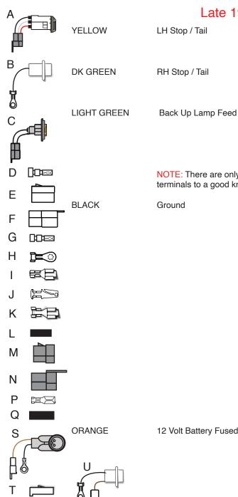
Route this wire to the LH tail lamp area, cut to length, install terminal I and plug into the empty cavity of connector M as shown on sheet 4. Do not plug your new stop/turn signal lamp pigtail A in yet, as the black ground wire circuit must be completed first.
